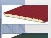
**CF Fluted Wall Panel** – The ribbed profile of the CF Fluted wall panel provides bold vertical lines complimentary to almost any commercial or industrial building. Inverted ribs in the profile enhance the high-tech industrial look. The interior skin has a Mesa profile. The CF Fluted panel offers a maximum R-value of up to R-42.9.
