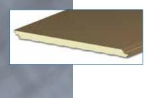
**Architectural Wall Panel** – The Architectural wall panel employs a flat appearance providing a monolithic look that is ideal for high-profile architectural applications. Both the interior and exterior skins are stucco embossed and the interior skin has a Mesa profile. The Architectural wall panel offers R-Values up to R-28.6.
