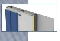
HPCI Barrier™ Wall Panel – The HPCI Barrier metal wall panel is an air, water, thermal and vapor barrier panel that can be used behind any type of façade. Installed in a horizontal orientation, completely outside of structural supports, there are no thermal bridges to reduce energy efficiency. The interior profile is Mesa. R-values of up to R-28.6 can be achieved with the HPCI Barrier Wall Panel.
